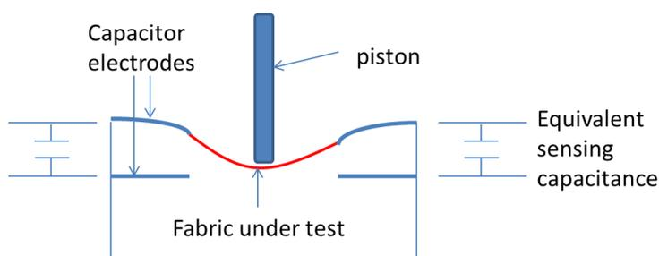
**Figure1.** Schematic of a capacitive multi-axial tensile testing device
