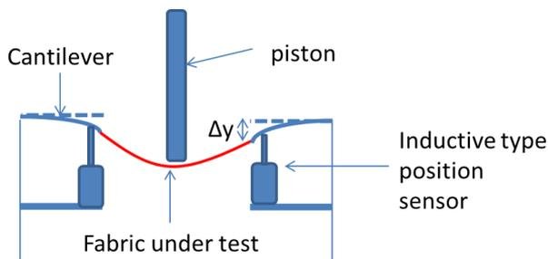
**Figure2.** Schematic of an inductive multi-axial tensile testing device
