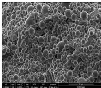
**Figure 2.** SEM image of the photochromic dye capsules obtained by spray drying
