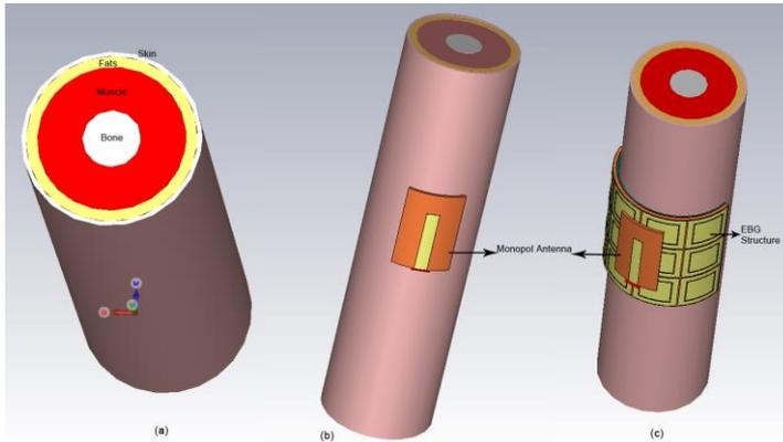
**Figure 3.** (a) Human body model, (b) A monopole antenna in direct contact with the human body and (c) Addition of EBG structure between the antenna and the human body
