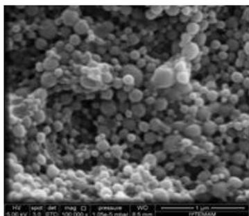
**Figure 1.** SEM image of the photochromic dye capsules obtained by solvent evaporation
