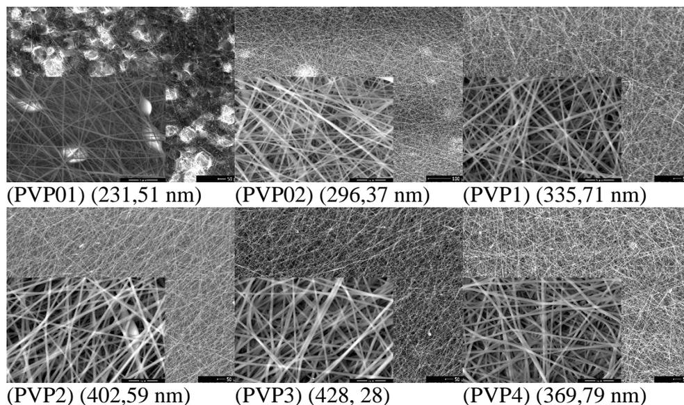
**Figure 1.** SEM images (1.000x-15.000x) of PVP nanofiber samples produced with various CEO concentrations
