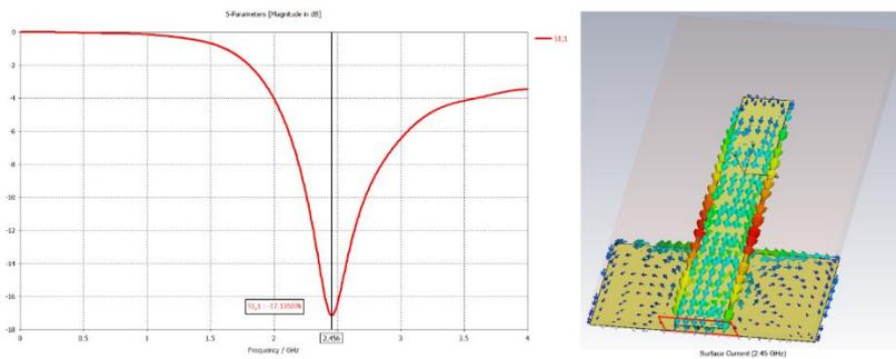
**Figure 2.** (a)  $S_{11}$  parameters graphic and (b) Surface currents
