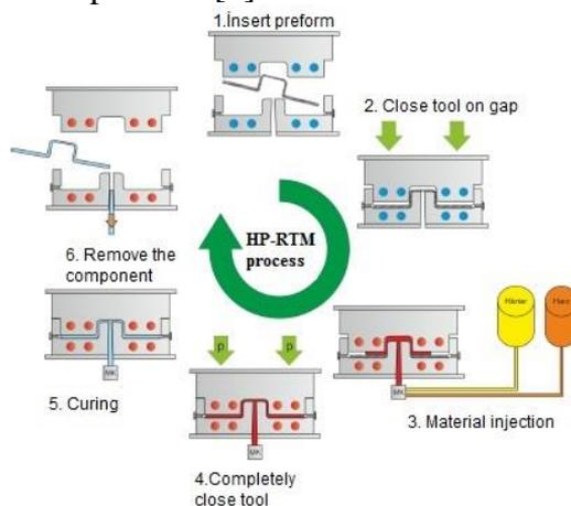
**Figure 1.** Schematic representation of the RTM method [6]
