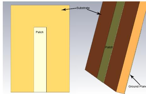
**Figure 1.** Electro-textile based monopole antenna design
