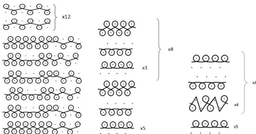
**Figure 1.** Stitch diagrams of designed sandwich knitted structures
