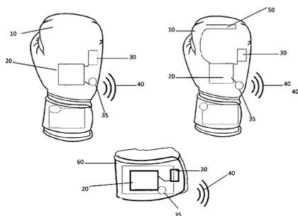
**Figure 2.** Boxing glove with accelerometers
