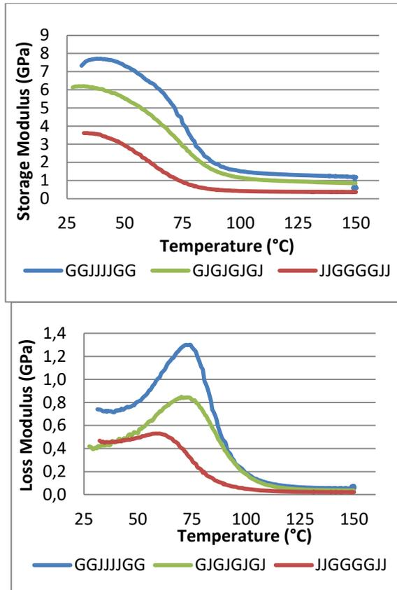
**Figure 1.** (a) Storage modulus, (b) loss modulus results of hybrid composite samples
