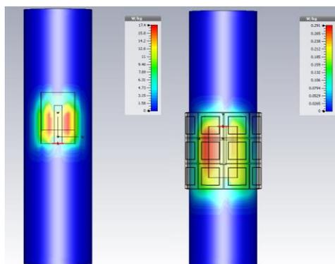
**Figure 4.** (a) SAR value obtained in direct contact (b) SAR value obtained when EBG structure was placed between human body and antenna
